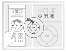
To set local time adjust time with "▲" "▼" button. To set local time press "◄" "▶" to change from hours to minute.
