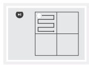
Press to wake up V8s, then press to start classic cleaning. The robot will clean in random and finish cleaning when the battery low.
